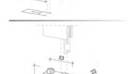
bottom / upper leveller diameter mm 34 - M6 threaded setting mm 30
