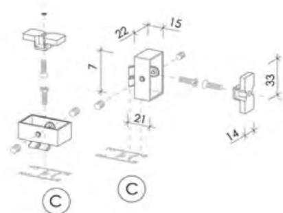
middle joint for levelling of profile C
