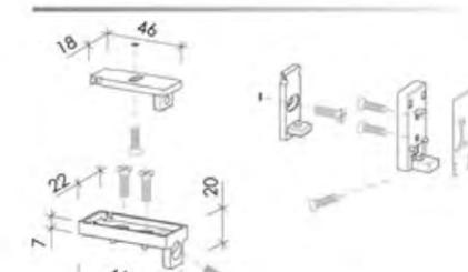
adjustable leveller for profile A - B (setting mm 23 )
