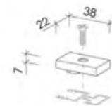
wall or ceiling joint for profile C
