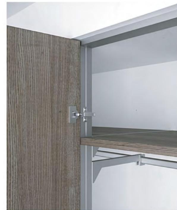
*Hinges can be mounted on the interior profile with mounting plate of 28 mm and the classical shelf shoulders or in alternative a rack can be placed on the back. The posterior profile fits a wooden or glass back (with seals). The cross profile is made ready to screw ties for the eccentric fixing of the tops and the bases of the wardrobes.*
