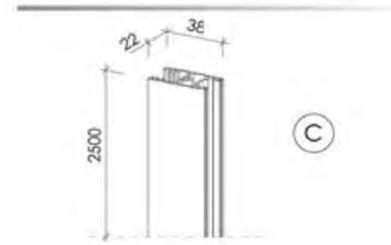
aluminium profile D 22x38x3000 mm for back cupboard's panel thickness mm 6
