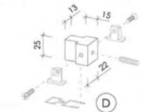
shelf joint or hinge fixing (with profile B)
