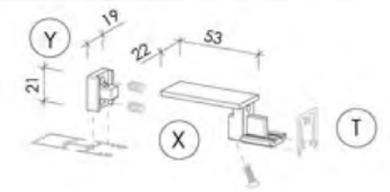
Y joint + J joint to fix D profile with cross profile T
