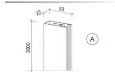
aluminium profile B 22x53x3000 mm with groove to fix hinges & supports for shelves
