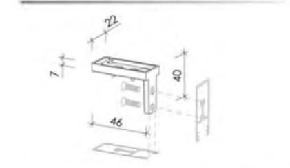
wall or ceiling fixing joint ( profile A - profile B )
