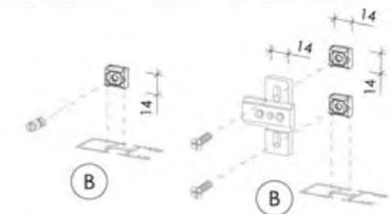
fixing joint for back profile D and cupboard's base/top
