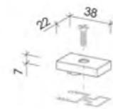
wall or ceiling joint for profile C
