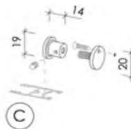
Y joint + W joint for middle fixing of cross profile T
